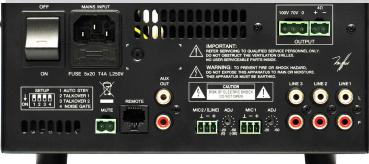
Self-powered mixer including an integrated media player and 5 external audio inputs: 3 x LINE ST, 1 MIC/LINE and 1 MIC. It features a 120W powered output that supports both low  $(4 \Omega)$  and high impedance (70V, 100V)loudspeaker lines. It also includes a 2 level priority system (paging, emergencies, etc.), auto stand-by mode, AUX OUT and an additional remote control port to manage the source selection and output volume by means of WPm series wall panels.
